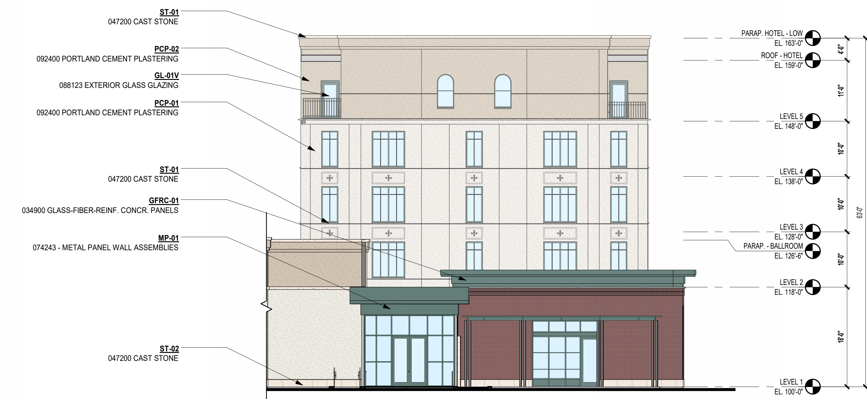
FACADE MATERIAL CALCS_ELEVATION - CONVENTION 03 ENTRY SCALE: 3/32" = 1'-0"
