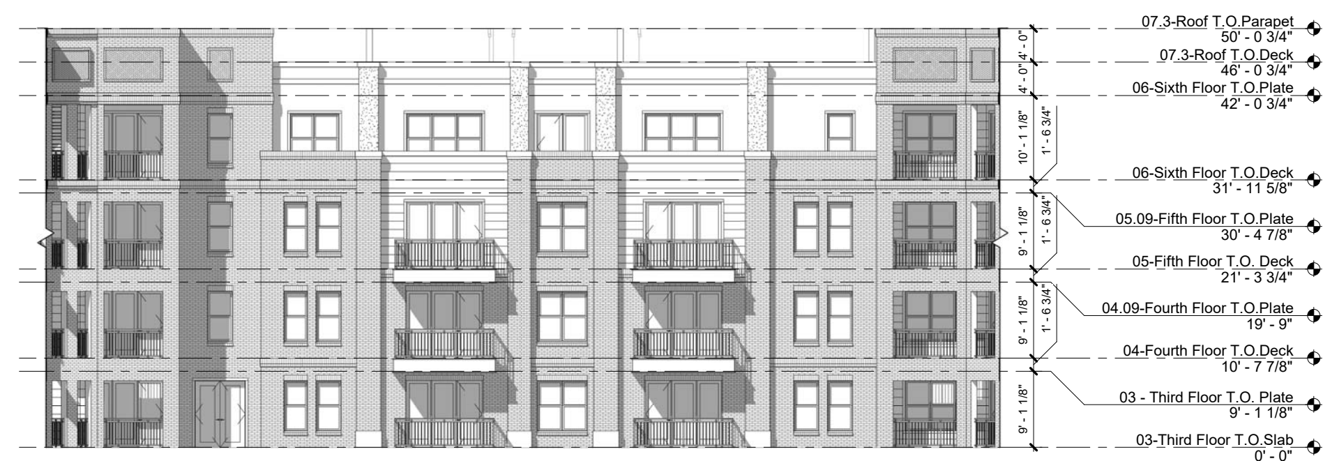
07 IL BUILDING - COURTYARD SOUTH ELEVATION 1/16" = 1'-0"
