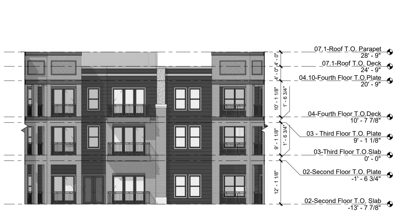
03 IL BUILDING - PODIUM COURTYARD EAST ELEVATION 1/16" = 1'-0"
