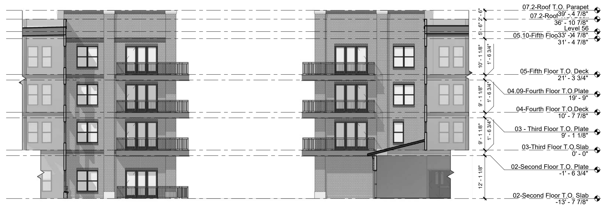
01 IL BUILDING - CLUBHOUSE COURTYARD EAST ELEVATION 1/16" = 1'-0"
