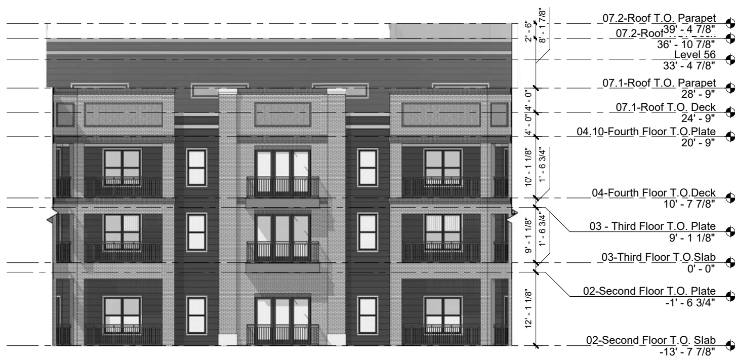
04 IL BUILDING - PODIUM COURTYARD SOUTH ELEVATION 1/16" = 1'-0"
