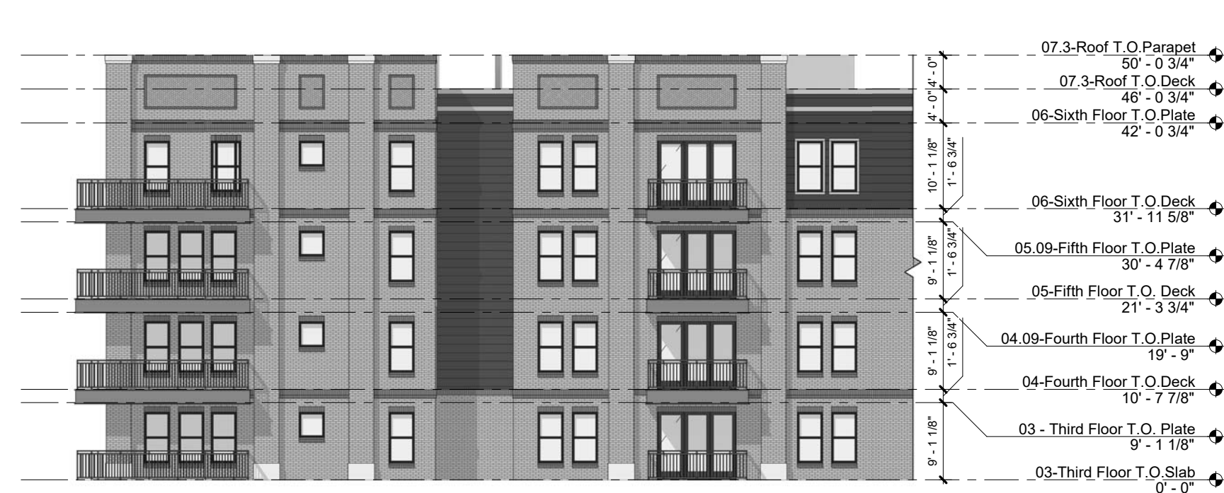
04 IL BUILDING - EAST ELEVATION 1/16" = 1'-0"
