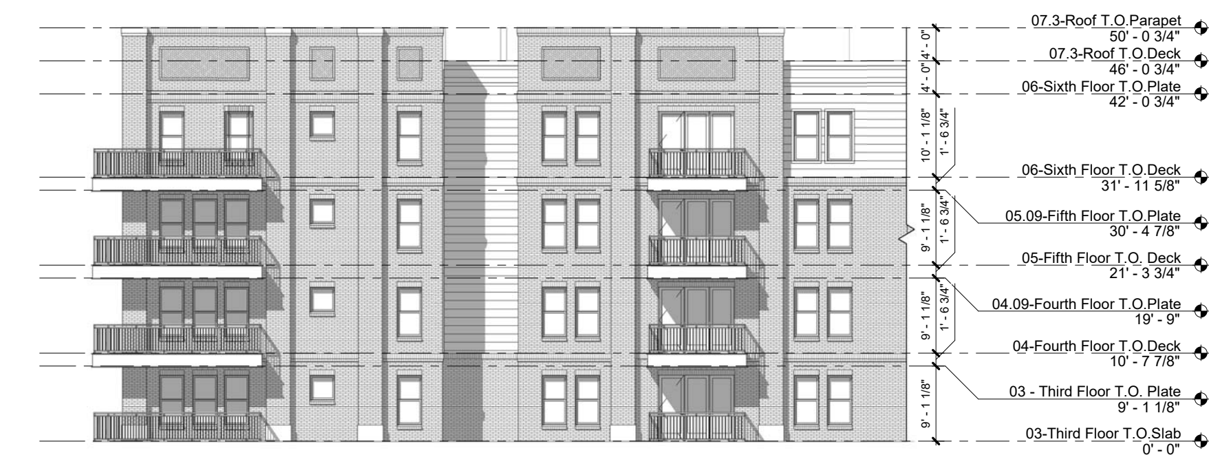
04 IL BUILDING - EAST ELEVATION 1/16" = 1'-0"
