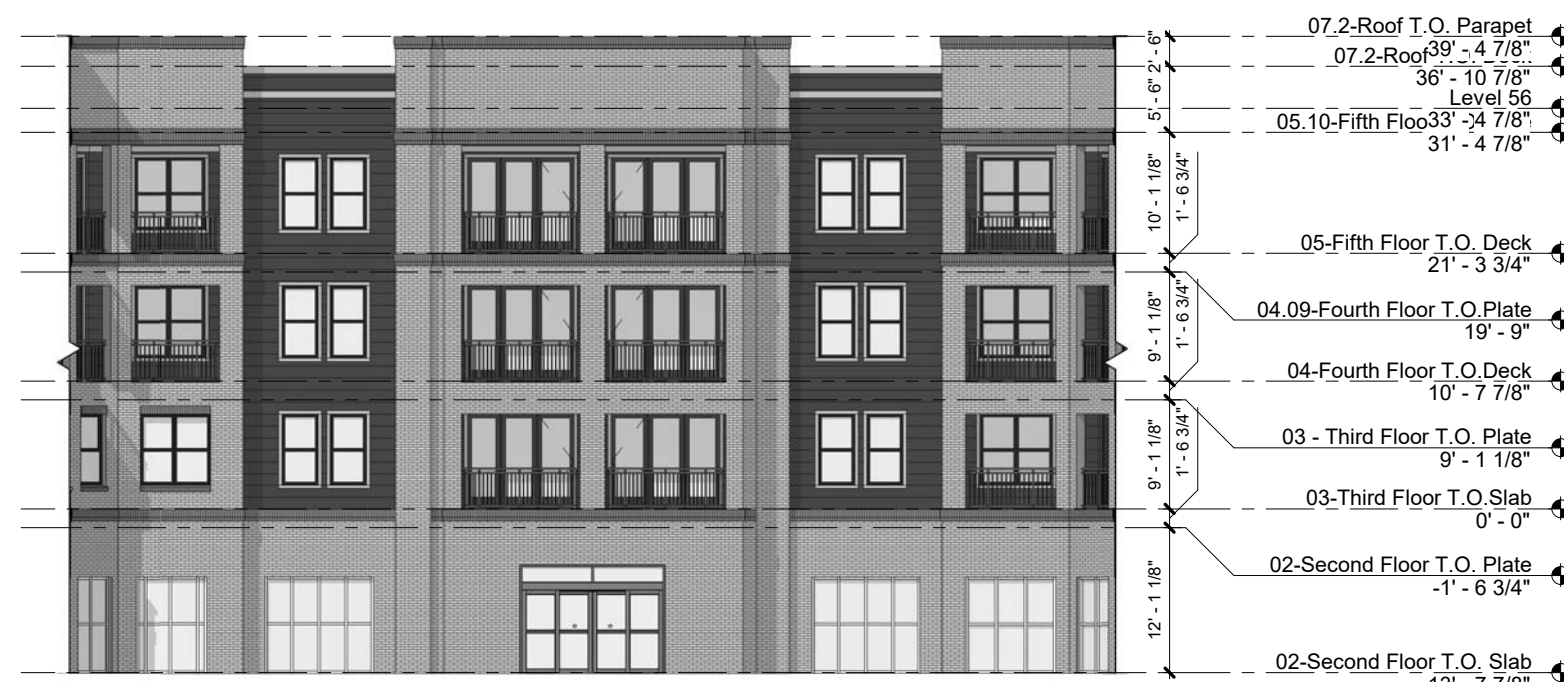
03 IL BUILDING - CLUBHOUSE COURTYARD WEST ELEVATION 1/16" = 1'-0"
