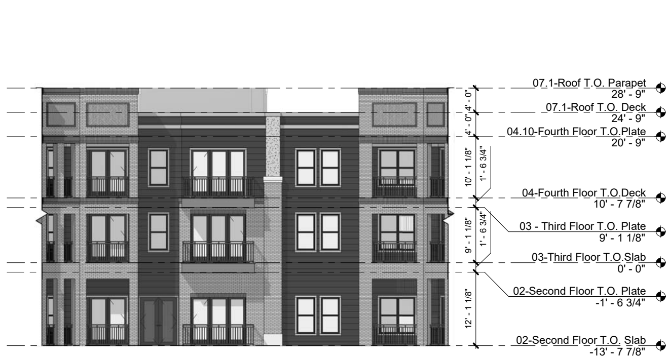
03 IL BUILDING - PODIUM COURTYARD EAST ELEVATION 1/16" = 1'-0"
