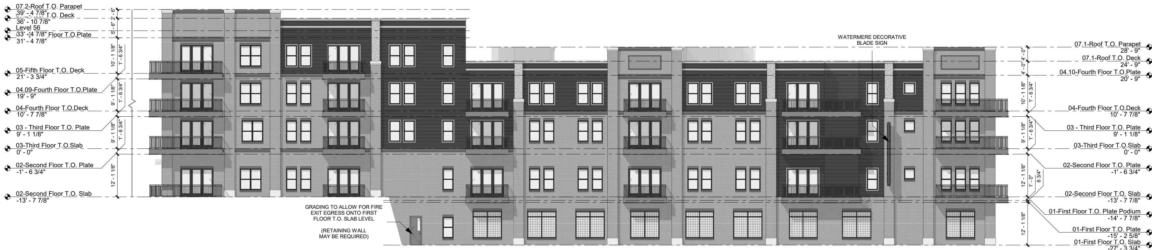
01 IL BUILDING - EAST ELEVATION CONT. 1/16" = 1'-0"
