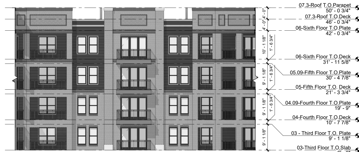
08 IL BUILDING - COURTYARD WEST ELEVATION 1/16" = 1'-0"
