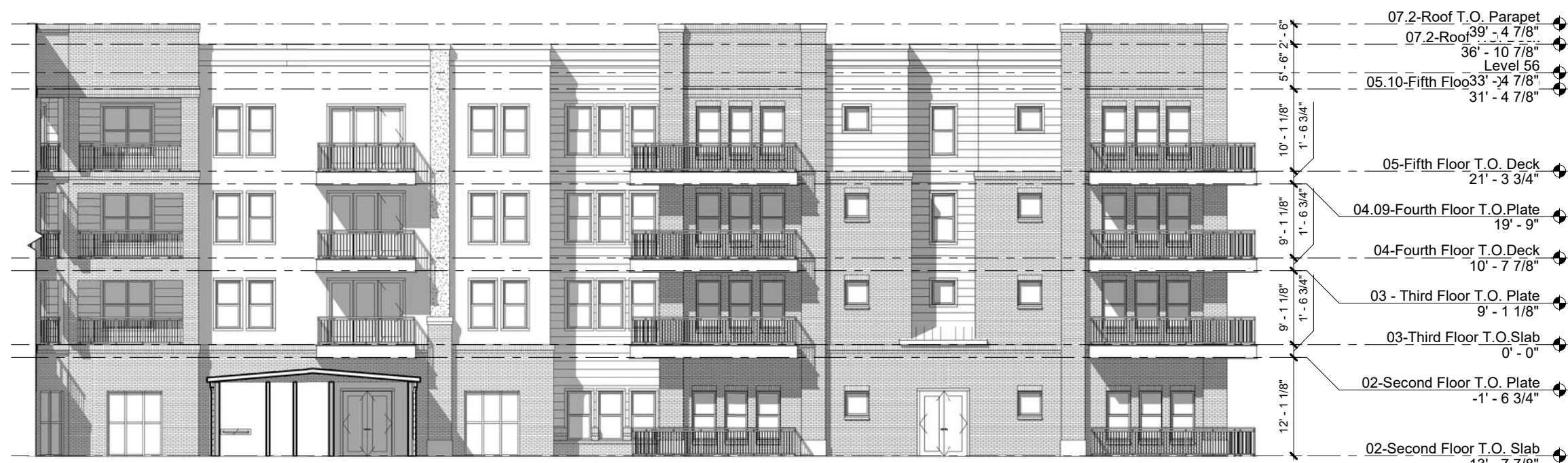
04 IL BUILDING - CLUBHOUSE COURTYARD NORTH ELEVATION 1/16" = 1'-0"
