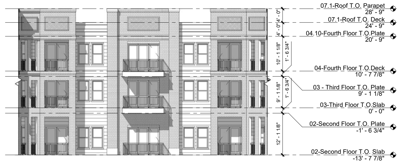
06 IL BUILDING - PODIUM COURTYARD NORTH ELEVATION 1/16" = 1'-0"
