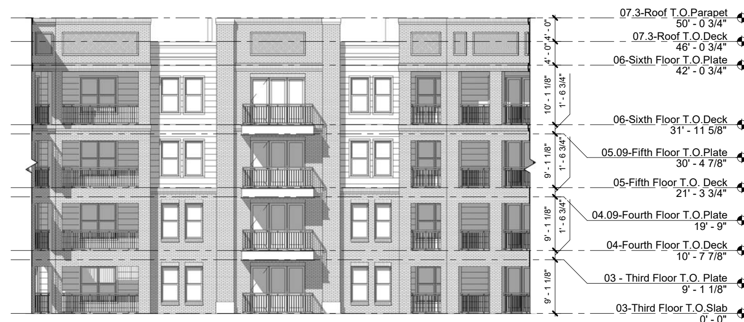
08 IL BUILDING - COURTYARD WEST ELEVATION 1/16" = 1'-0"
