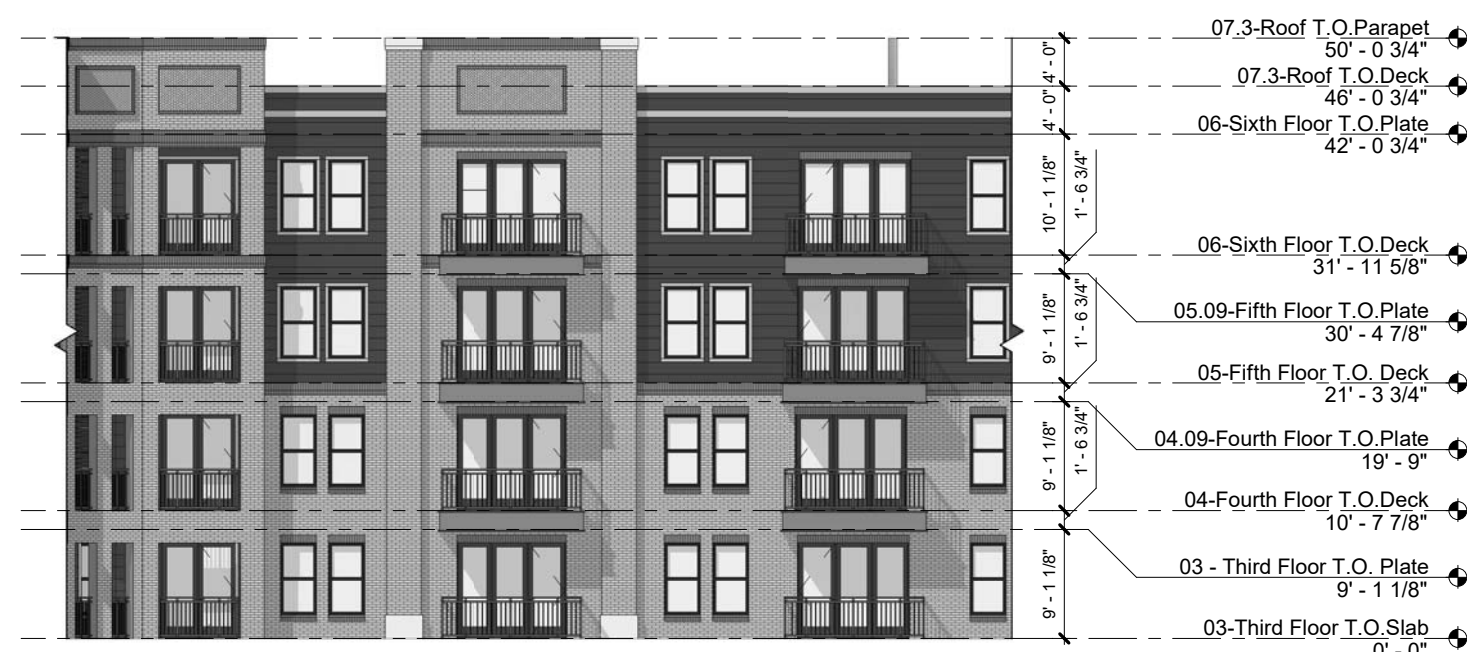
05 IL BUILDING - COURTYARD EAST ELEVATION 1/16" = 1'-0"
