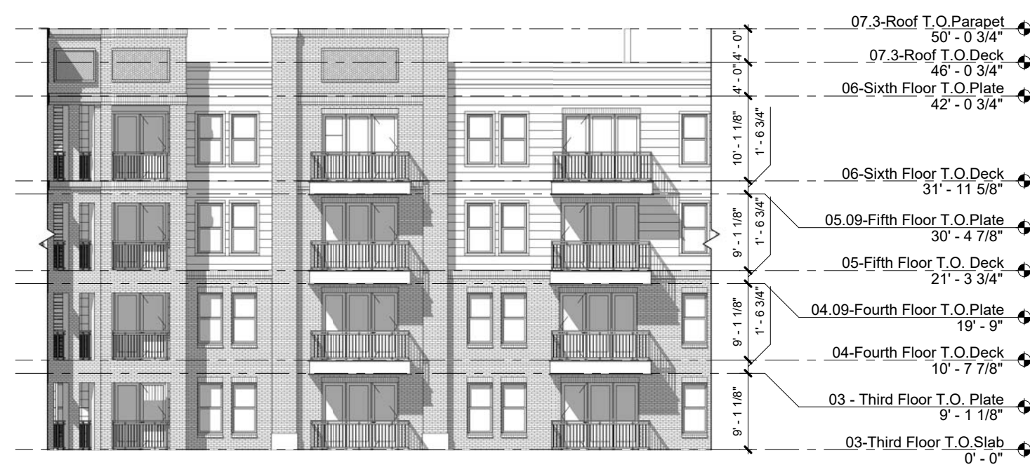
05 IL BUILDING - COURTYARD EAST ELEVATION 1/16" = 1'-0"
