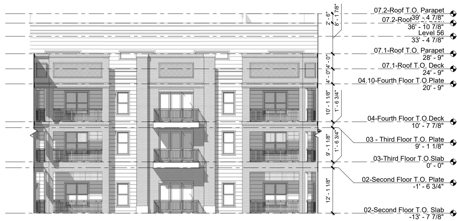
04 IL BUILDING - PODIUM COURTYARD SOUTH ELEVATION 1/16" = 1'-0"
