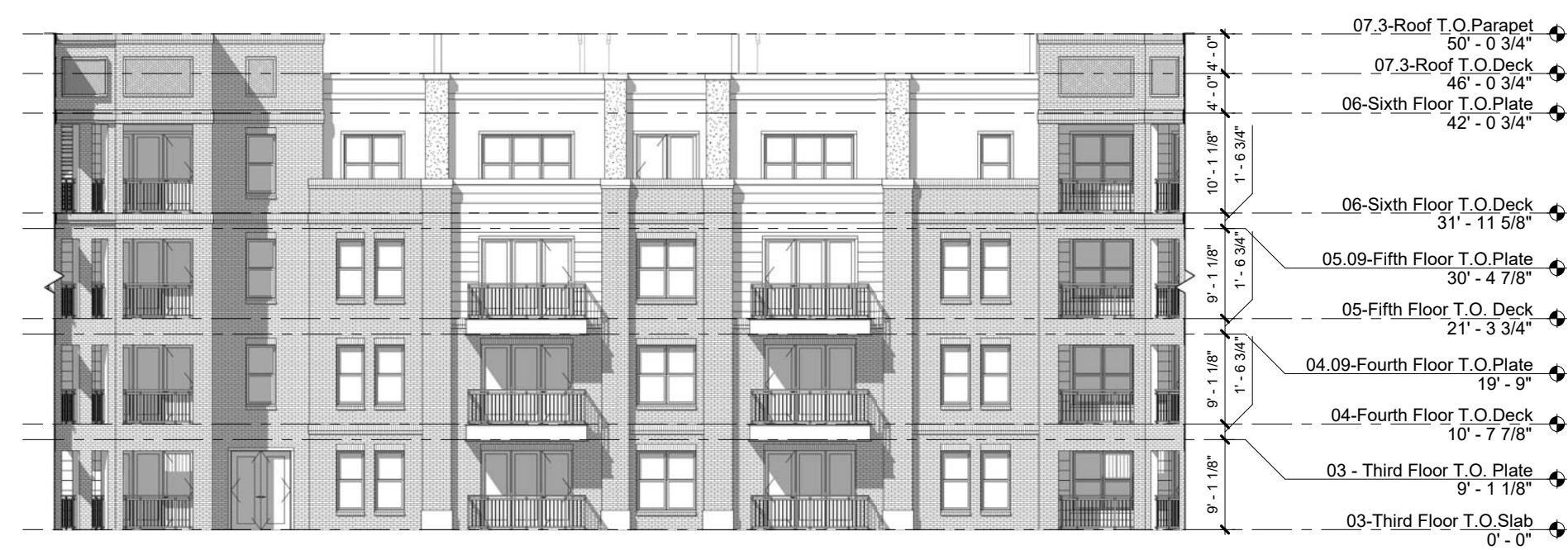
07 IL BUILDING - COURTYARD SOUTH ELEVATION 1/16" = 1'-0"
