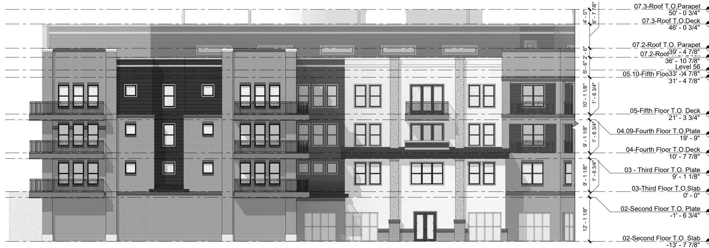
02 IL BUILDING - CLUBHOUSE COURTYARD SOUTH ELEVATION 1/16" = 1'-0"
