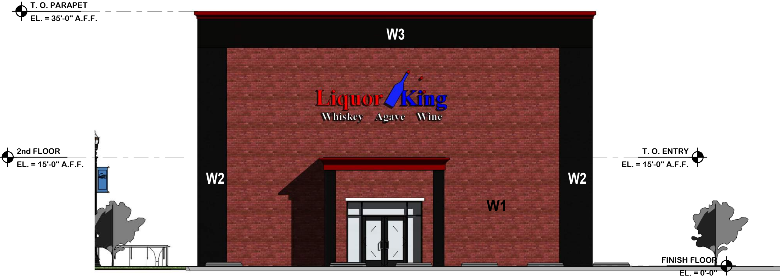
4 EXTERIOR ELEVATION BUILDING 1 SCALE: 1/8" = 1'-0"
