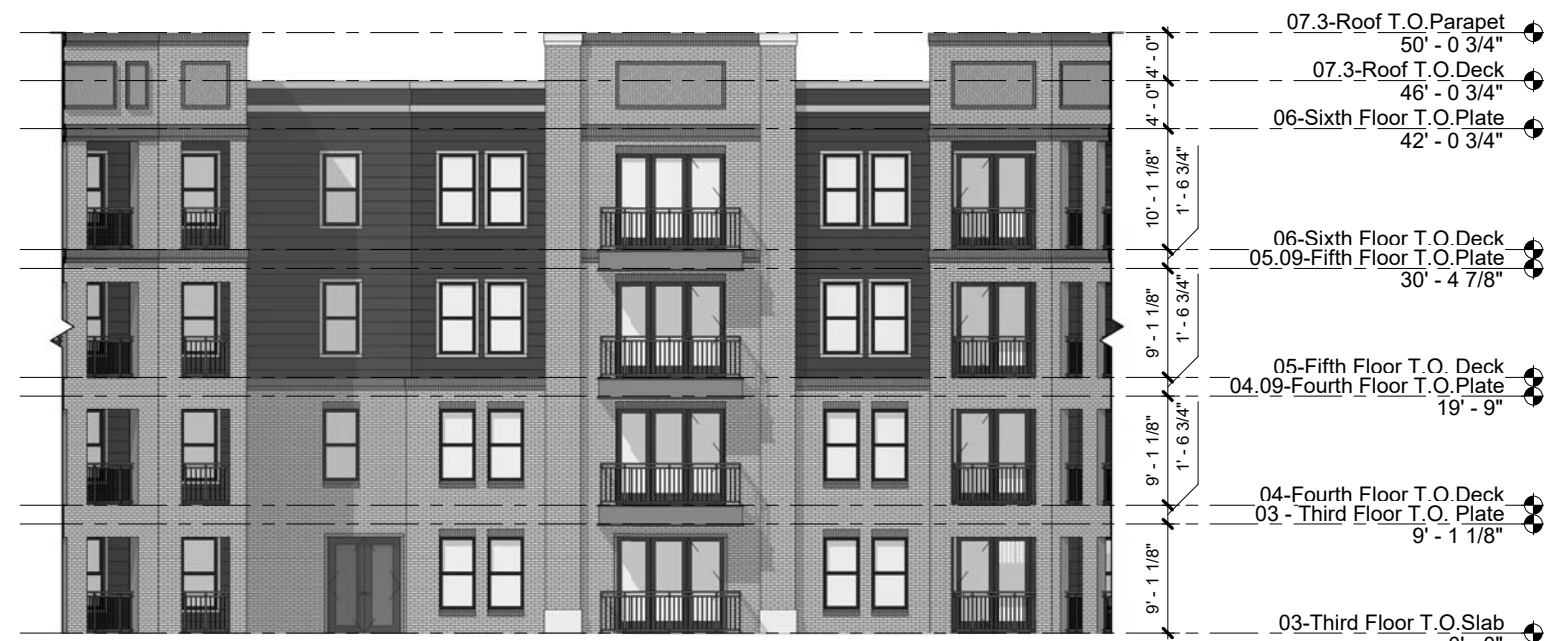
09 IL BUILDING - CLUBHOUSE COURTYARD NORTH ELEVATION 1/16" = 1'-0"
