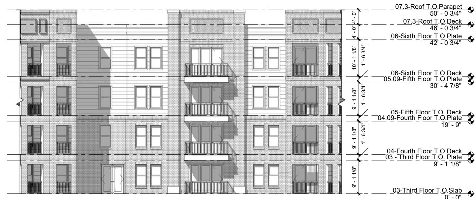
09 IL BUILDING - COURTYARD NORTH ELEVATION 1/16" = 1'-0"
