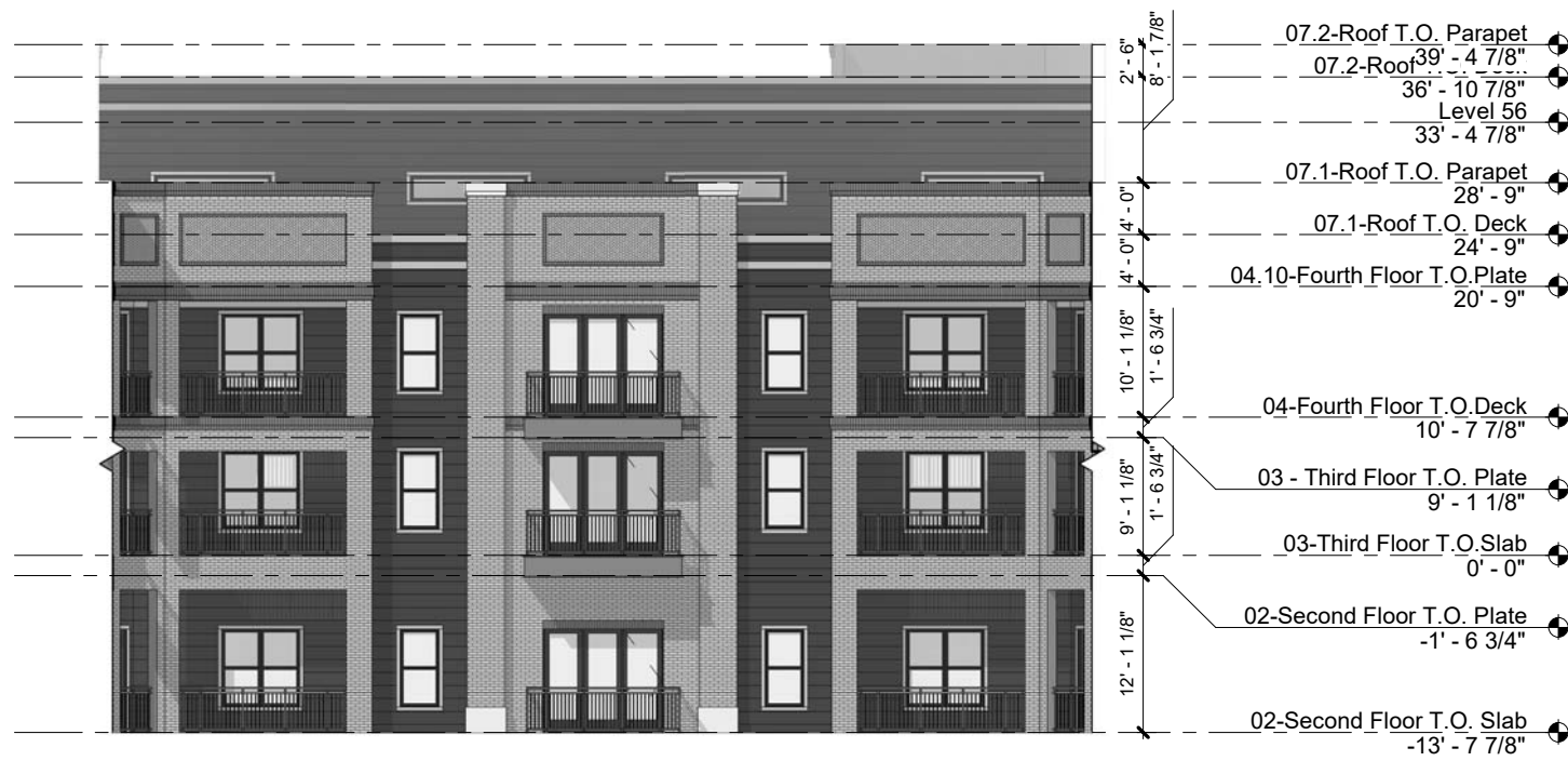
04 IL BUILDING - PODIUM COURTYARD SOUTH ELEVATION 1/16" = 1'-0"
