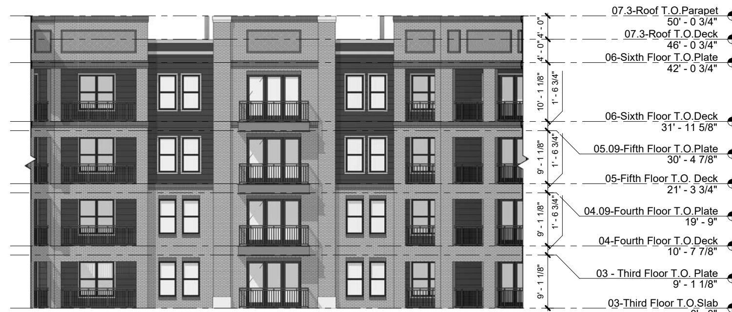
08 IL BUILDING - CLUBHOUSE COURTYARD WEST ELEVATION 1/16" = 1'-0"
