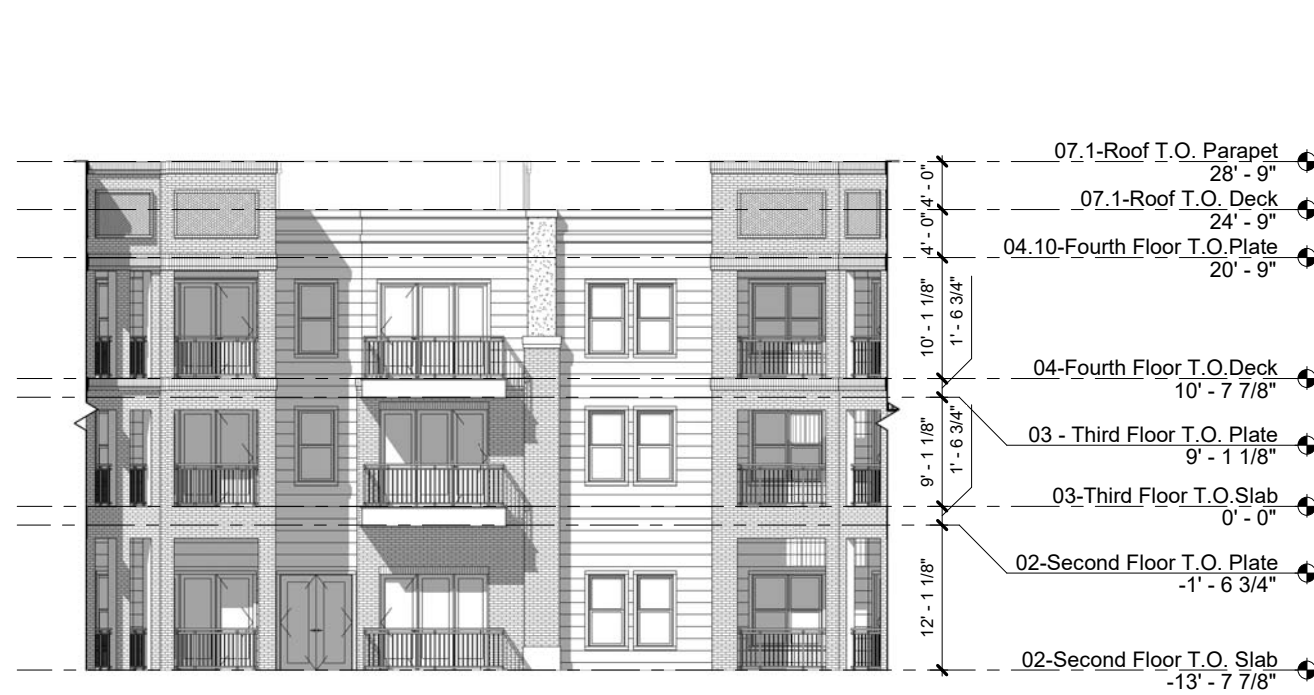
03 IL BUILDING - PODIUM COURTYARD EAST ELEVATION 1/16" = 1'-0"
