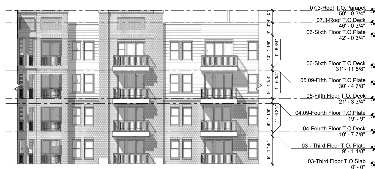
05 IL BUILDING - COURTYARD EAST ELEVATION 1/16" = 1'-0"
