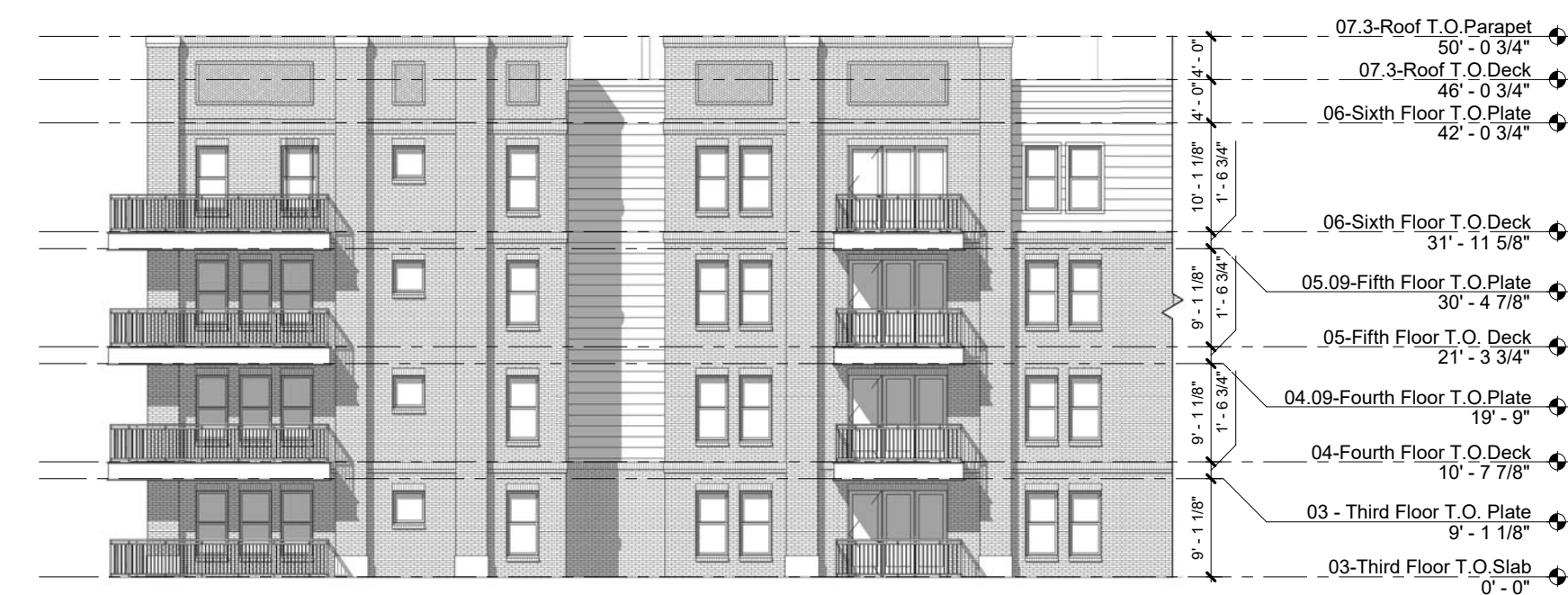
04 IL BUILDING - EAST ELEVATION 1/16" = 1'-0"
