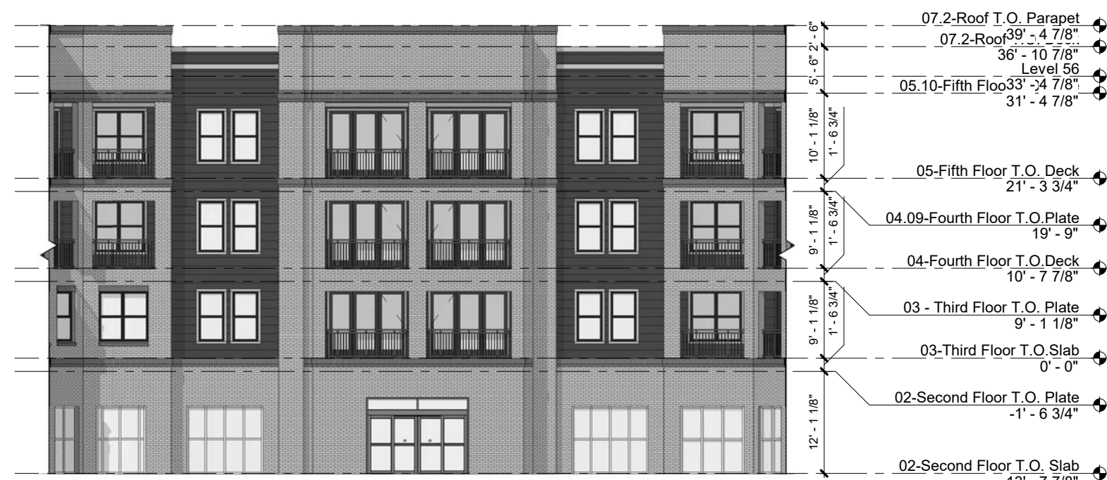
03 IL BUILDING - CLUBHOUSE COURTYARD WEST ELEVATION 1/16" = 1'-0"
