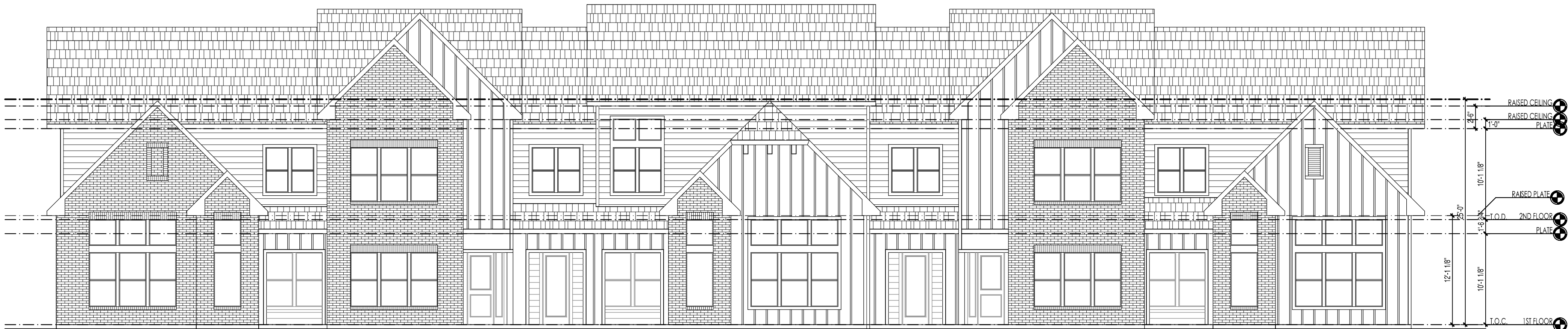
3 ELEVATION - NORTH SCALE 1/8"=1'-0" MATERIAL PERCENTAGES MASONRY (BRICK/STUCCO/STONE) 0% EC SIDING 100% MATERIAL PERCENTAGE TOTAL 100%
