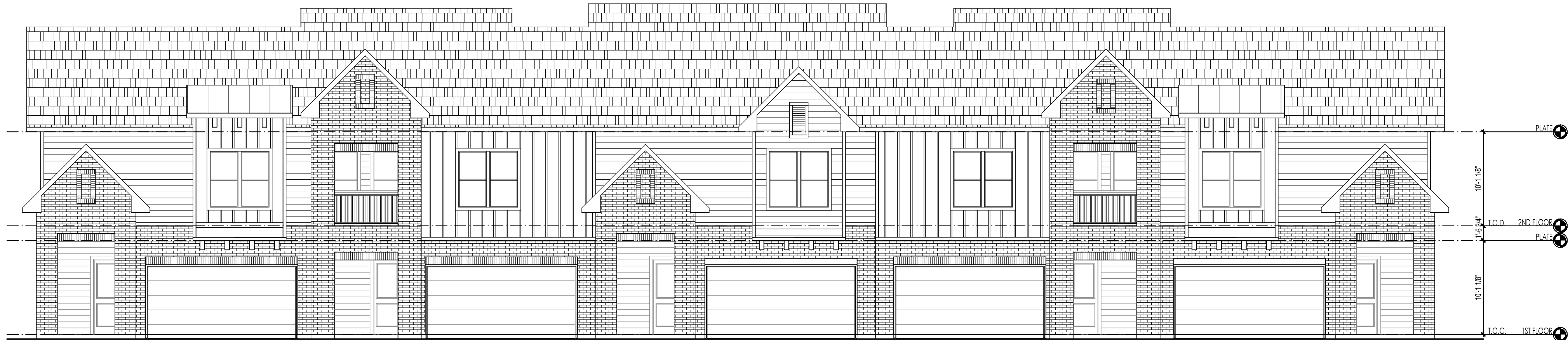
1 ELEVATION - SOUTH SCALE 1/8"=1'-0" MATERIAL PERCENTAGES MASONRY (BRICK/STUCCO/STONE) 50% EC SIDING 50% MATERIAL PERCENTAGE TOTAL 100%
